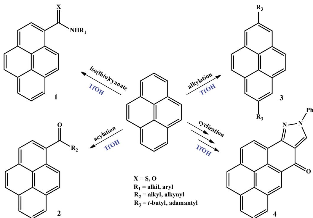
Scheme 1: Application of triflic acid in the synthesis of pyrene derivatives.
