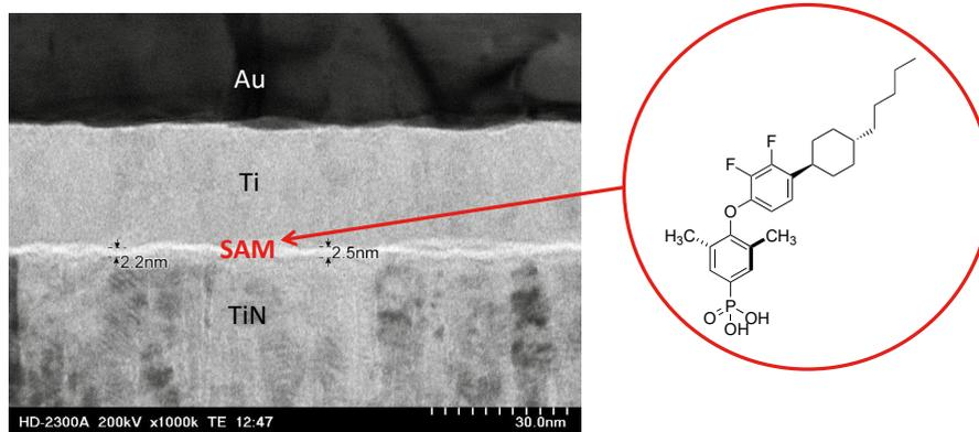
Figure 1: STEM micrograph of a cross section through a solid state tunnel junction (TiN/SAM/Ti/Au) containing a SAM composed of a dipolar phosphonic acid.
