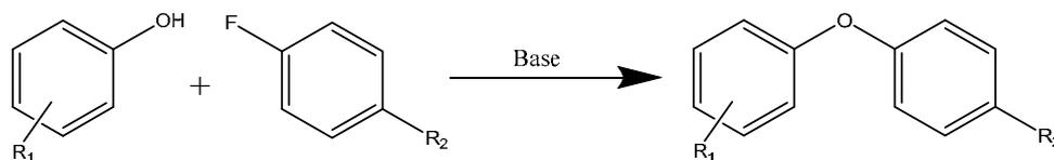
Figure 1:  $S_NAr$  reaction of phenol derivatives with fluorobenzenes.
